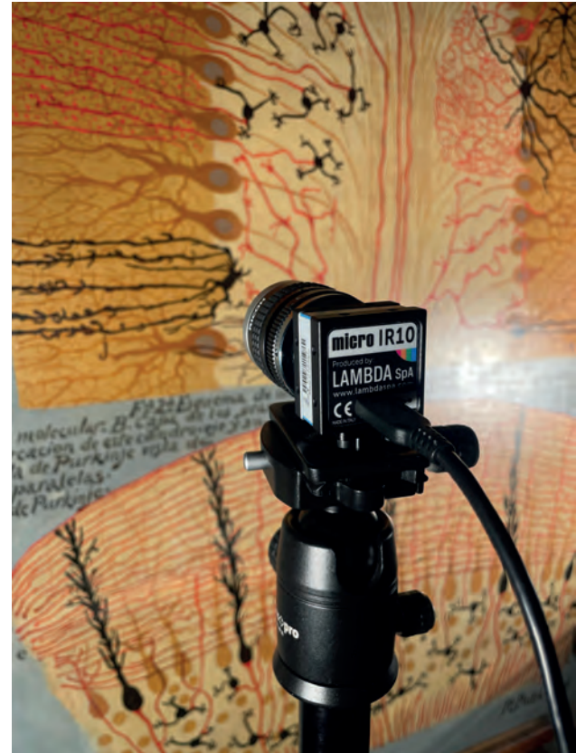
Technical examination of one of the works by Ramón y Cajal and Padró y Pedret using infrared reflectography. Silvia G. Fernández-Villa
