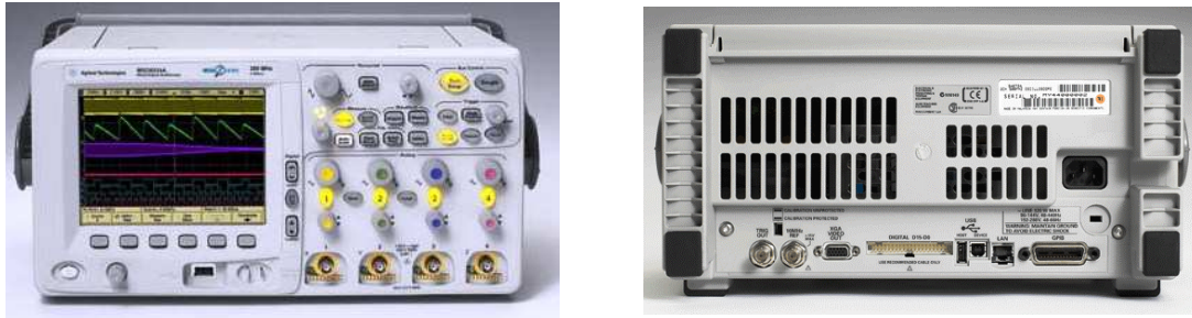
Fig. 5.3: Agilent Oscilloscope model DSO6104A. Left, front panel; Right, Rear panel.
