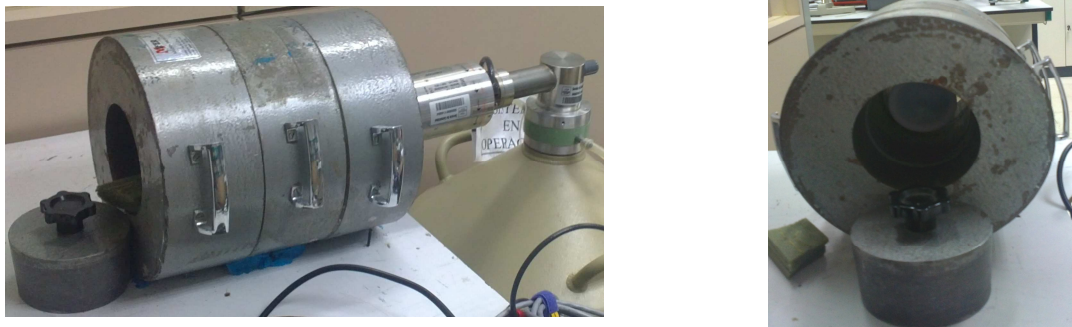
Fig. 2.9: Lead shielding. Left, how the shielding covers the PopTop and the end cap. Right, the space to put material is appreciated.
