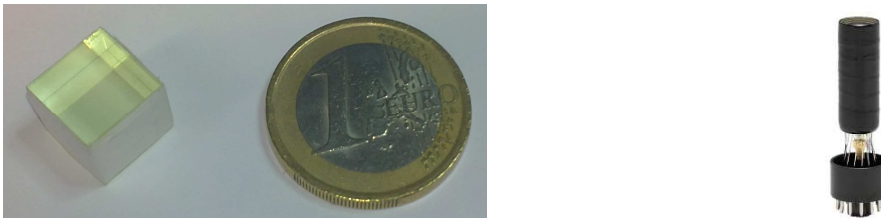
Fig. 3.7: Left, LuAG:Pr scintillator crystal by side of a one-euro coin. Right, photo of a R5320 PMT.
