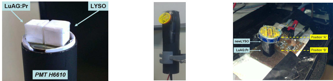
Fig. 5.6: Configurations tested. Left, side-by-side configuration in the PMT. Middle, phoswich coupled to the PMT with a gamma point-like source. Right, the phoswich coupled to SiPM in a black box.
