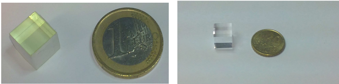
Fig. 5.2: Left, the LuAG:Pr scintillator. Right, LYSO crystal. Both are cubes of 1\text{ cm}^3 .
