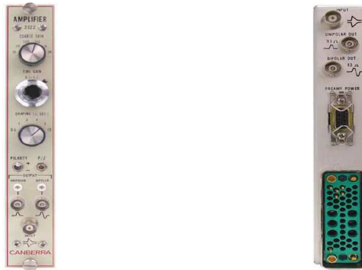
Fig. 2.13: Canberra Amplifier model 2022. Left, frontal panel. Right, Rear panel.
