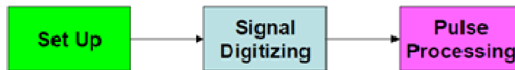
Fig. 5.1: Scheme of the stages to characterize a phoswich: first chose the right set up, then use an appropriate digitizing system and lastly explore pulse processing strategies.
