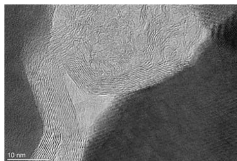
Fig. 7. TEM micrograph of ex-CNF graphite sheets between 8YSZ grains in 8Y-2CNF-1600.
