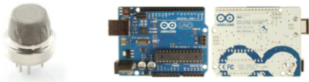
Fig. 8. The MQ-4 gas sensor (left) and Arduino Board (right).
