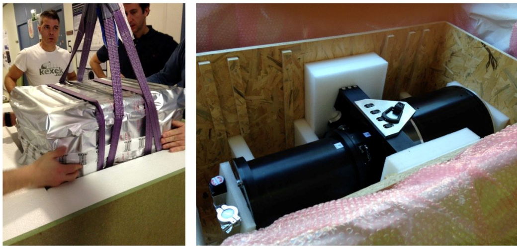
Figure 7: Left: Introducing a packed VPH grating in its transport box. Right: Camera-cryostat assembly in its transport box.
