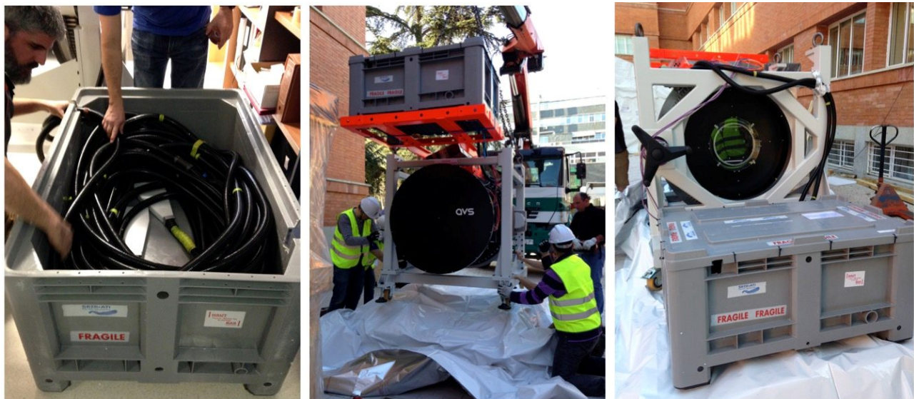
Figure 6: Left: Fiber bundles in its transportation box. Center: FC subsystems and fiber bundle box handled to its transportation box. Right: FC subsystems in its transportation box in shipping configuration.
