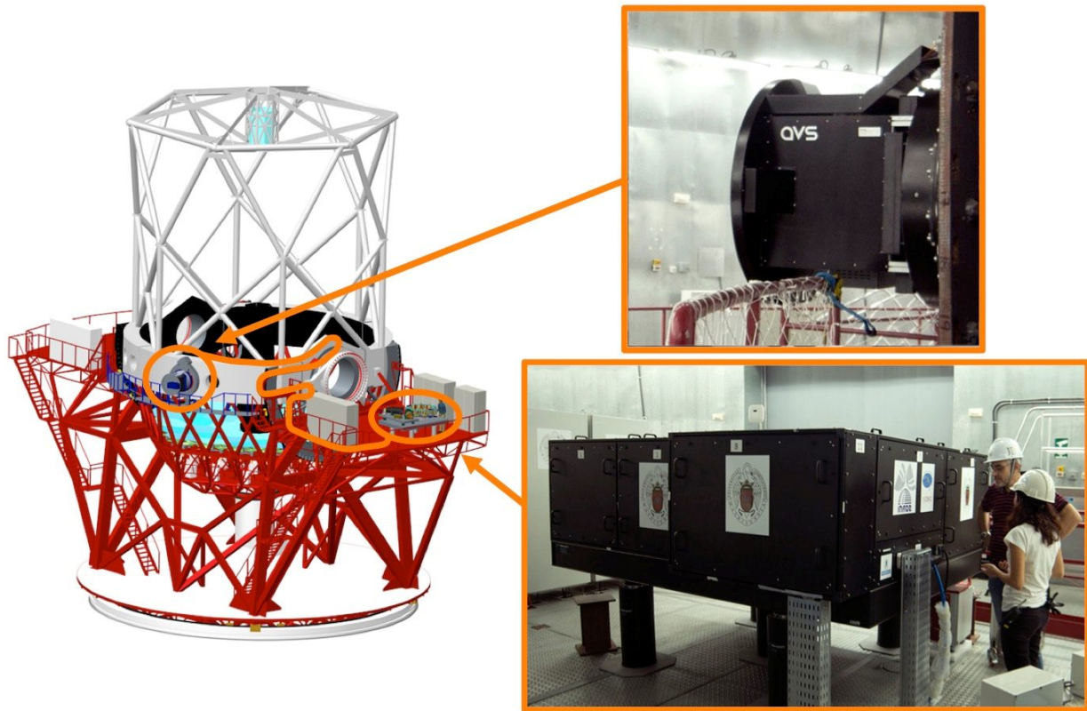
Figure 1: On the left, a GTC 3D model with MEGARA Folded Cassegrain subsystems integrated at FC-F focal station and MEGARA spectrograph at the Nasmyth A platform. On the right, views of the real MEGARA subsystems already integrated at the GTC.
