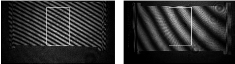
Figure 2: The set of 5 fringes images for the 1.5_F691@0016_MN_DSC_190101_074147_5.stk file (run 5r01, cell #5, laser MN, Temperature gradient build-up step).
