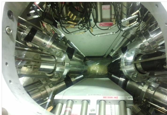
Figure 4.7: Setup picture of the target area. - Photograph of the setup in the target area showing some of the BGO-shielded Ge clovers and the \text{LaBr}_3(\text{Ce}) detectors placed in a close-geometry configuration around the target position. The yellow structure corresponds to the target.
