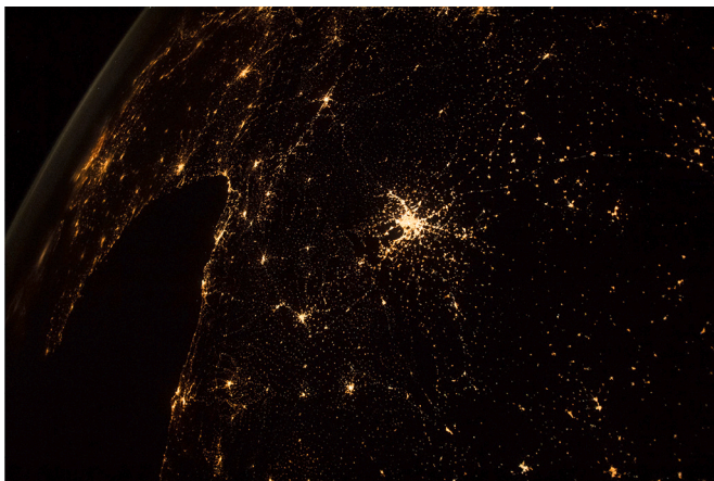
Fig. 7. Original JPG image of Spain used as an exemplar. Madrid (the spider-like lit area) looks to be saturated, although this is not actually the case. This is only one of the reasons not to use JPG images, although geometrically it is equivalent to the RAW image, colours, relative intensities, and other issues like gamma correction mean that this is not recommended.
