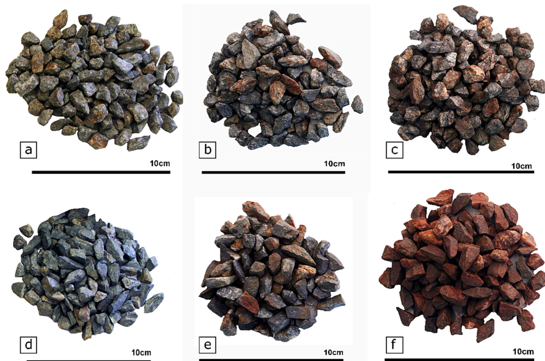
Fig. 5. Examples of schist 6/12 aggregate (a–c) and amphibolite 6/12 aggregate (d–f), before (a and d) and after the freeze-thaw (b and e) and thermal stress (c and f) tests [50].
