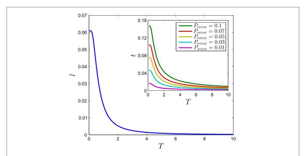
**Figure 3.** Amount of spatial correlations  $\bar{I}$  along the t–T line corresponding to constant error probability  $P_{\text{error}} = 0.1$ . We see the rapid decreasing of  $\bar{I}$  as T increases (J = 1 and  $\gamma_0 = 4/3$  in units of  $\omega$ ). The inset shows t–T isolines for various values of the error probability  $P_{\text{error}}$ , which increases with both t and T.
