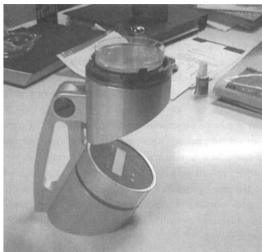
Fig 3 MAS-100 Air Sampler (Merck) and Sabouraud irradiated agar plates used in our hospital for sampling high-risk areas.
