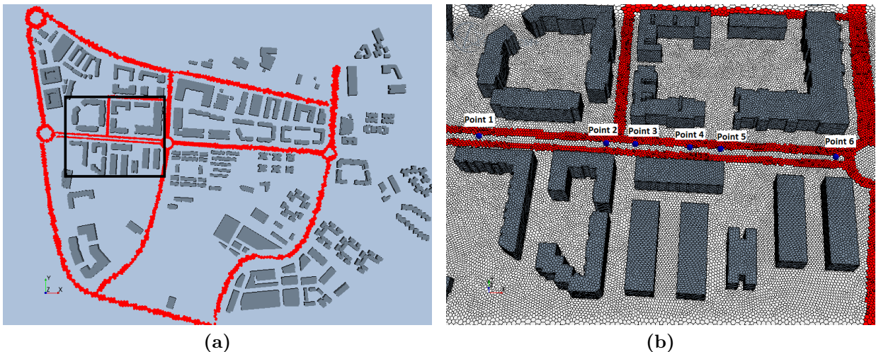
Figure 1: (a) Geometry of the computational domain and the research area limited by the black square. (b) Mesh of the research area and location of the measurements points.
