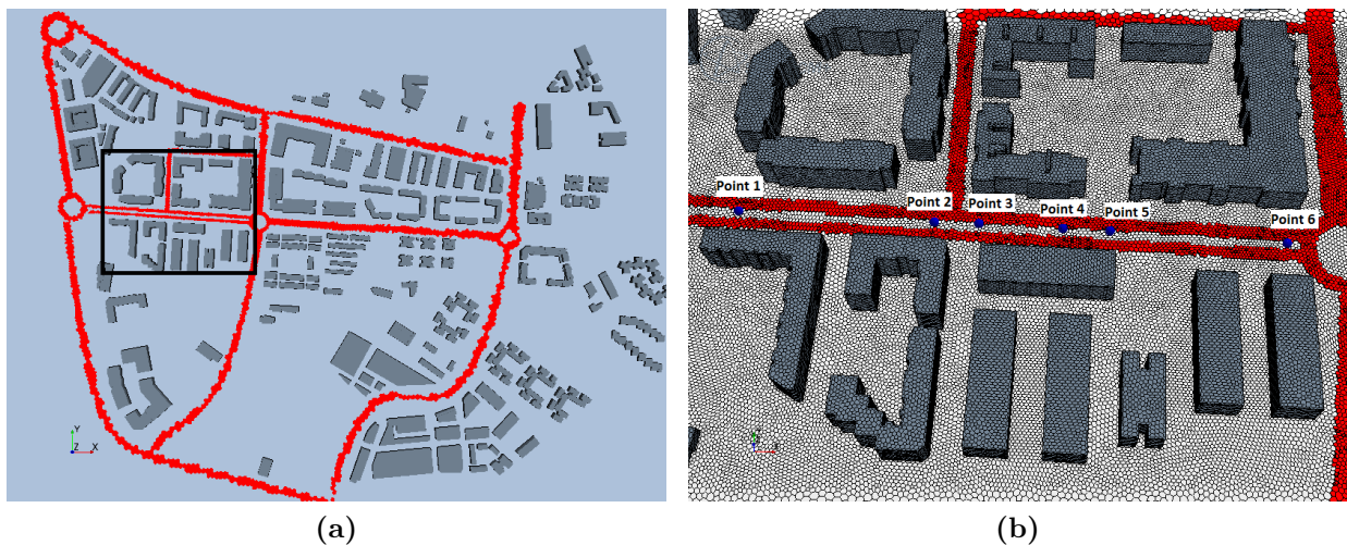
Figure 4.2: (a) Geometry of the computational domain and the research area limited by the black square. (b) Zooming in on the meshed research area and location of the measurements points.
