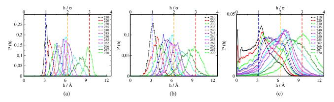
FIG. 3. System size analysis of thickness distributions at the basal plane. (a) Probability distribution of the global film thickness  $h_{1/4}$ . (b) Probability distribution of the partial film thickness  $h_{1/4}$ . (c) Probability distribution of the local order parameter  $h(\mathbf{x})$ . Dashed vertical lines show the film thickness in units of the molecular diameter. Results are shown for temperatures in the range from T = 210 K to T = 271 K, with color code as indicated in each panel.
