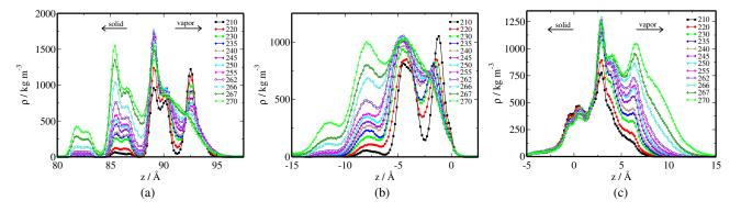
FIG. 1. Density profiles of liquidlike molecules for the basal interface as measured relative to (a) the laboratory reference frame, (b) the f-v surface, and (c) the i-f surface. Since the liquidlike layer has finite thickness, the profiles vanish at the solid phase to the left and the vapor phase to the right of the z axis.
