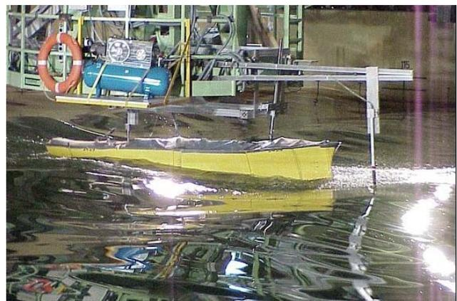
Fig. 1: A towed scaled replica at CEHIPAR
