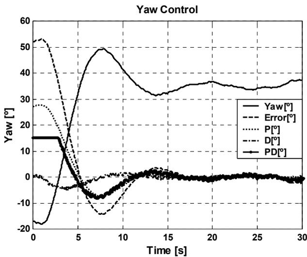
Fig. 10. Yaw control components.
