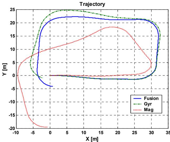
Fig. 7. Magnetic and Gyroscopic sensors fusion.
