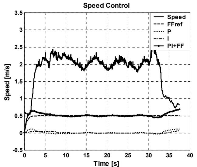
Fig. 11. Speed control components.
