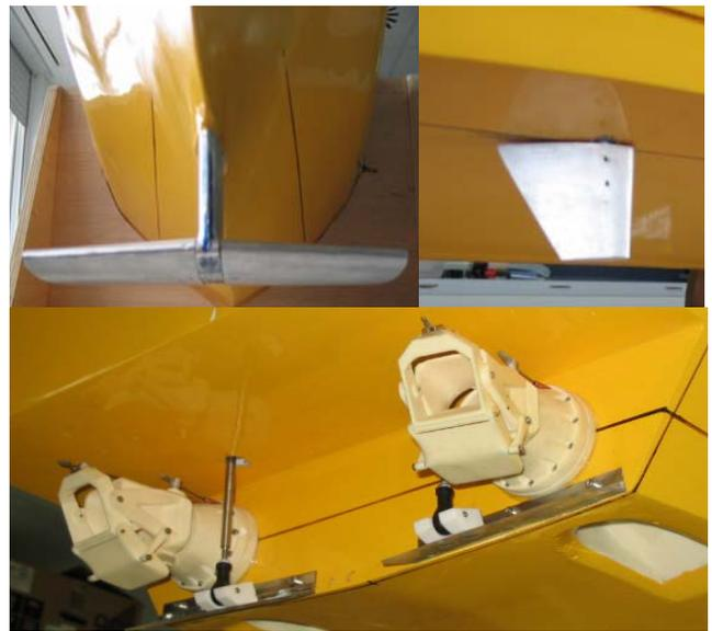
Fig. 4. Scaled actuators: T-Foil, Fins, Flaps and Jets.
