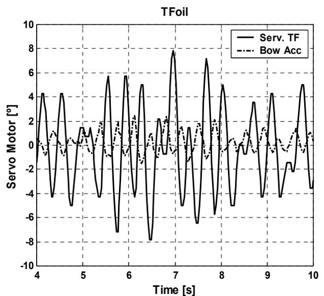
Fig. 12. T-Foil control action.
