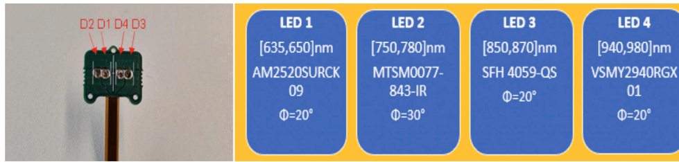
Fig. 6. Physical layout and identifiers of the four LEDs. Wavelengths (610, 740, 850, 940 nm) were selected for differential tissue penetration and melanin sensitivity. Emission angles ( \Phi = 20\text{--}30^\circ ) optimize targeting of digital arteries for high-quality photoplethysmographic signals.
