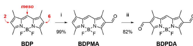
Scheme 3. Synthetic route towards BDPDA dopant. Reaction conditions: i. \text{POCl}_3 , DMF, DCE, 60 ^\circ\text{C} , 1 h; ii. \text{POCl}_3 , DMF, \text{CH}_2\text{Cl}_2 , reflux, 48 h.
