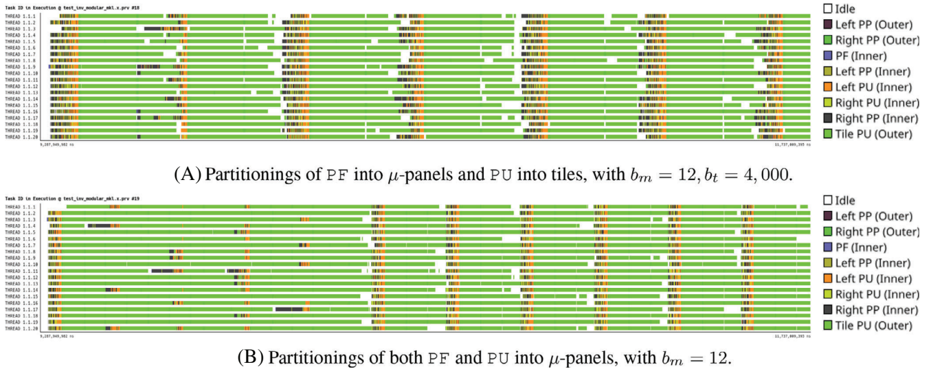
FIGURE 9 Traces of the first 0.5 s of the execution of the ATP GJE algorithms, with n = 16,000, b_p = 480 , and 20 cores on SKYLAKE
