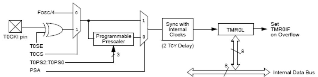
Note: Upon Reset, Timer0 is enabled in 8-bit mode with clock input from T0CKI max. prescale.
