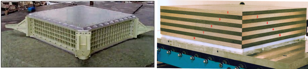
FIGURE 2.15: (Left) ECAL honeycomb structure. PMTs are installed on the squared holes. (Right) Distribution of the nine superlayers, with the fibers arranged in alternating directions.
