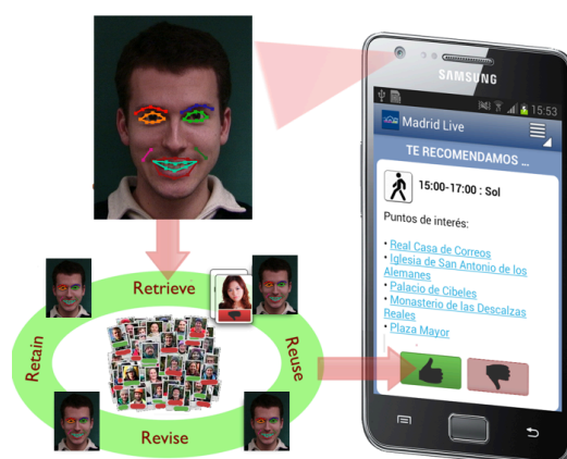
Figura 7.4: CBR process to detect a users' emotions from images of their face.
