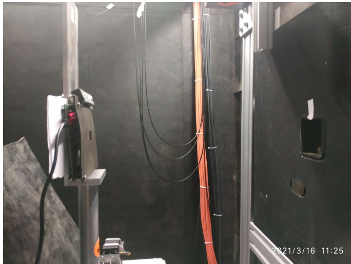
Figure 4.8: Setup for the irradiation of the FPGA at the ILL.
