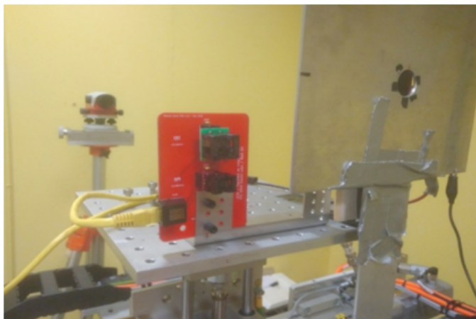
Figure 4.6: Setup for the irradiation of the nv-SRAM and FRAMs at the CNA.
