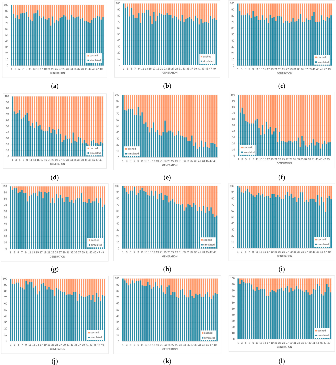
Figure 10. Simulated vs. cached circuit evaluations per generation for a population of 100 individuals and for SPICE-only optimization with NSGA-II, NSGA-III, and SPEA2, respectively, of the operational-amplifier topologies under test: (a–c) Miller-compensated differential amplifier; (d–f) Transistor-compensated differential amplifier; (g–i) folded-cascode op-amp; (j–l) Telescopic-cascode amplifier.
