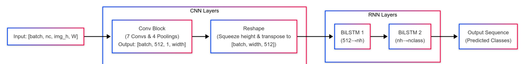
Figure 3. The CRNN model structure.
