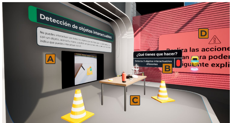
Fig. 3 Example of tutorial scenario. The figure represents the detection of interactable objects step ( TUTISEL ). The description panel can be seen in A . The task to be performed by the user is shown in B . C is the zone where the elements that the user must interact with to complete the task are located. D is the wall that blocks the user until the task is completed
