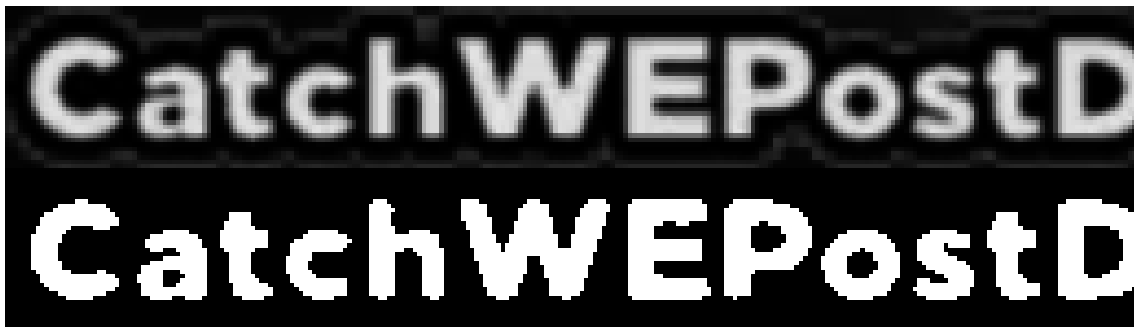
Figure 4.10: Top: Luminance map of a region. Bottom: Mask obtained from applying threshold to luminance map
