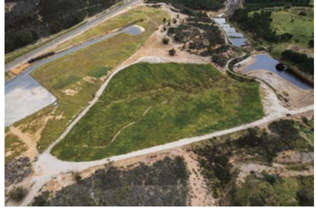
Figure 5. Aerial view of the intervention area of the LIFE RIBERMINE project after geomorphic remodelling, edaphic cover, and endemic re-vegetation.
