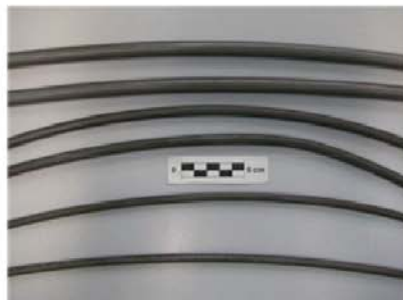
Figure 1: Wire rods of boron steel (30MnB5) drawn wire.
