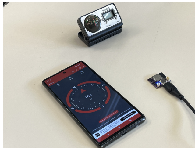
Figure 4.5: Relative positioning of the phone, compass, and sensor during the alignment experiment.
