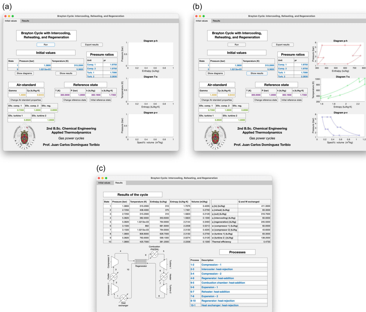
FIGURE 3 Brayton cycle with intercooling, reheating, and regeneration: (a) tab with the initial values obtained after running the application; (b) tab with the thermodynamic diagrams corresponding to the solved cycle (after pushing the “Show diagrams” button); (c) results tab with the thermodynamic properties of the cycle states, heats and works exchanged, and the thermal efficiency of the cycle.
