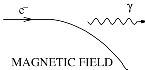
Figure 1.6: Schematic of curvature radiation [21].
