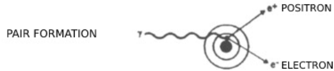
Figure 1.9: Schematic of classical pair production adapted from [22].
