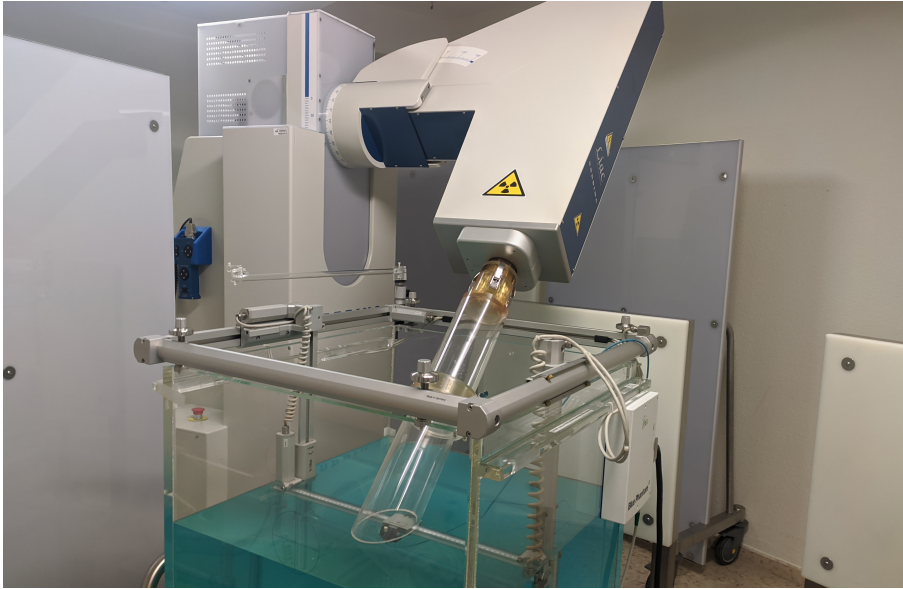
Fig. 1: Typical setup for determining output factors with a beveled applicator.
