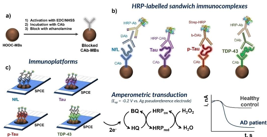
**Figure 1.** Schemes of the developed electrochemical immunoplatforms for the determination of NfL, Tau, p-Tau and TDP-43 involving the modification of MBs with CAbs (a), the formation of sandwich immunocomplexes labelled with HRP (b) and amperometric detection at SPCEs (c).
