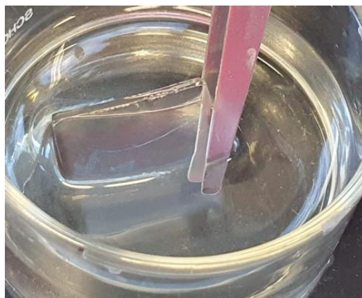
Figure 4.10. Photograph of a reference sample after 24 hours in basic water: in this reference sample HCL(jef) has been replaced by polyethylene glycol dimethacrylate (PEGDMA) in the same percentage by weight (15%).
