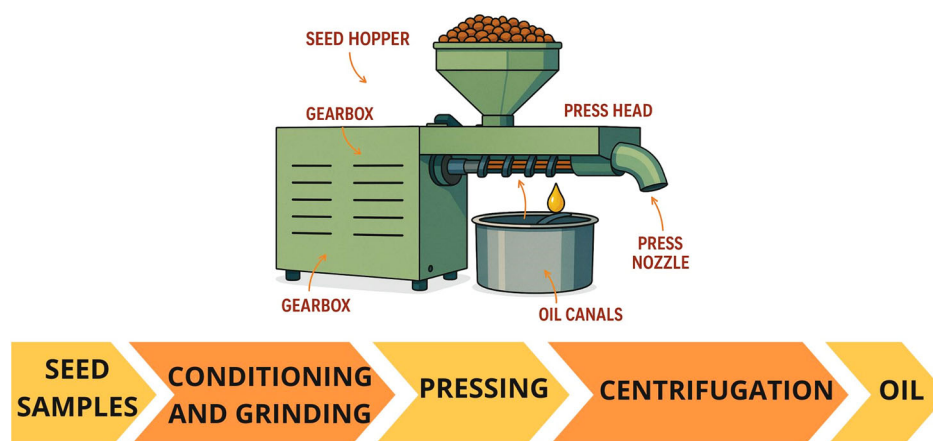
Figure 5. Flow chart of oil extraction through mechanical pressing.
