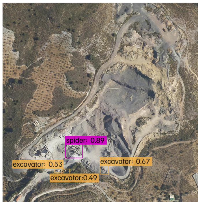
Figure 2. Examples of element detection within an aggregate quarry using computer vision.
