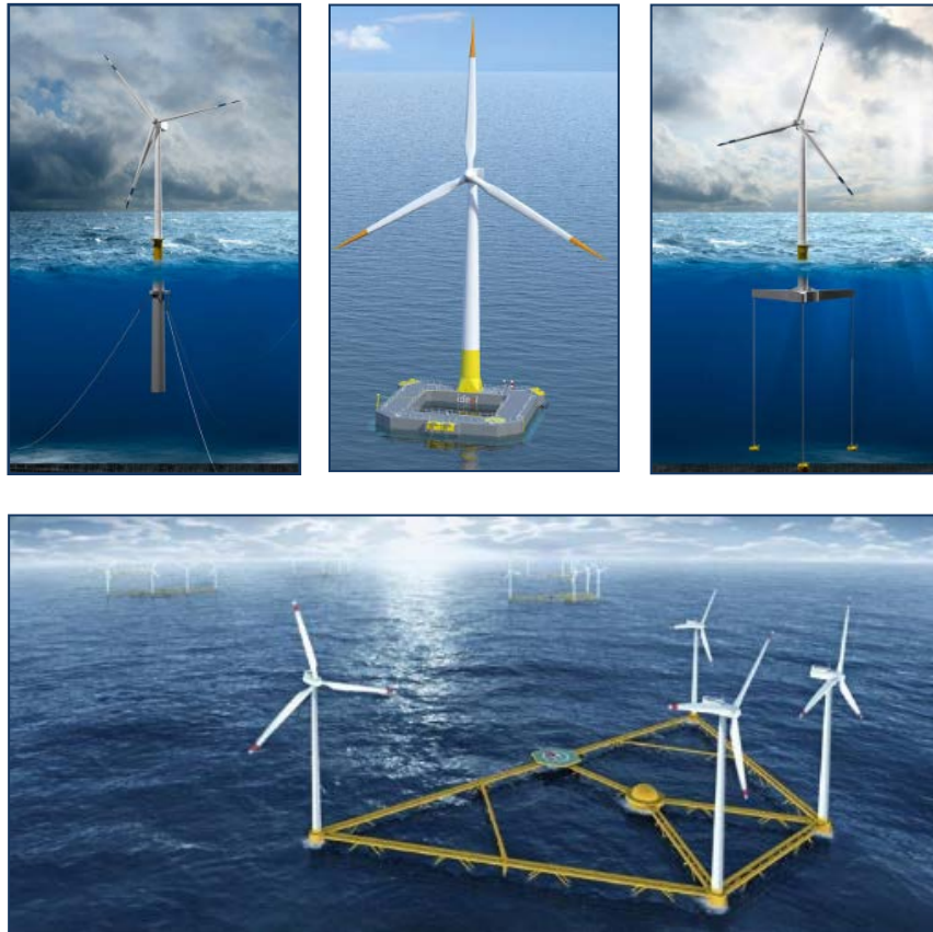
Figura 2-3. Soportes flotantes: spar, semisumergible, TLP y multi-turbina [11] [12] [13]
