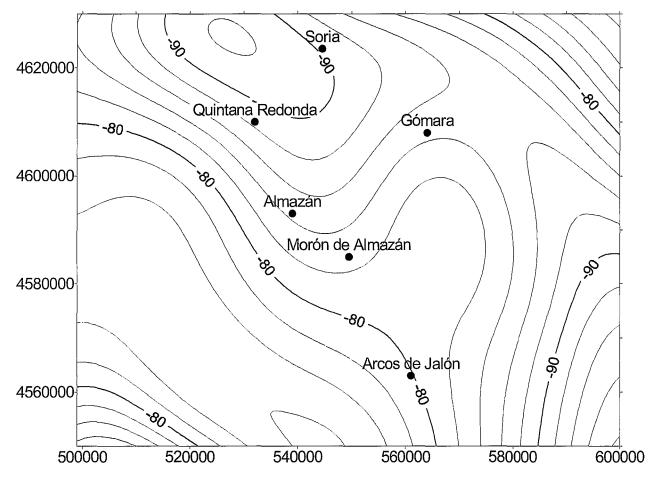
Figure 8.- Bouguer anomaly map showing the effect of the regional source isolated. Contour interval 2 mGal. UTM coordinates as in figure 2.
