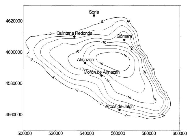
Figure 4.- Theoretical gravity anomaly map, showing the gravity effect of the sedimentary infill, using a density ranging at depth from 2.46 gr/ cc to 2.69 gr/cc. Interval 2 mGal. UTM coordinates as in figure 2.
