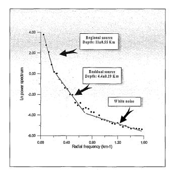
**Figure 7.-** Graph showing power spectrum versus radial frequency for the gravity map in figure 3. Three different sources, regional, residual and white noise are distinguished, and their mean depths have been calculated.
