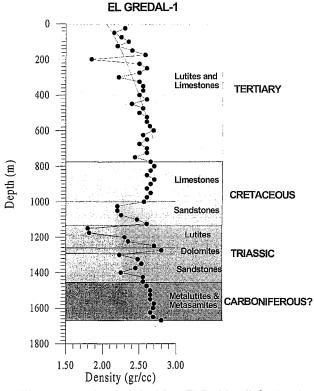
**Figure 5.-** Density log derived from El Gredal well. See location on figure 3. Black line between 0 and 700 m depth represents the least square fit to a quadratic function for depth variation density. The density obtained has been used for the computation of the gravity anomaly depicted on figure 4.
