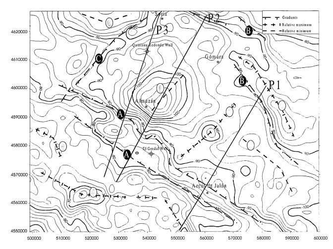
Figure 3.- Gravity anomaly map of the Almazán Basin. Contour interval 2 mGal. UTM coordinates as in figure 2. The location of the three gravity models is shown. Numbers and letters refer to features described on the text.
