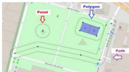
Figure 4: Location-based geometries. The red is POI, the blue is polygon and the purple is a path.
