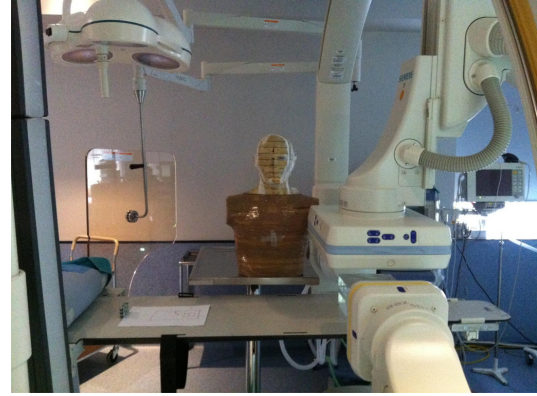
Fig. 1. Simulation of paediatric interventional cardiology procedures performed with the phantom. Three OSLDs were placed in the left eye. A 20 \times 20 \times 12 \text{ cm}^3 PMMA slab was used to simulate the paediatric patient.
