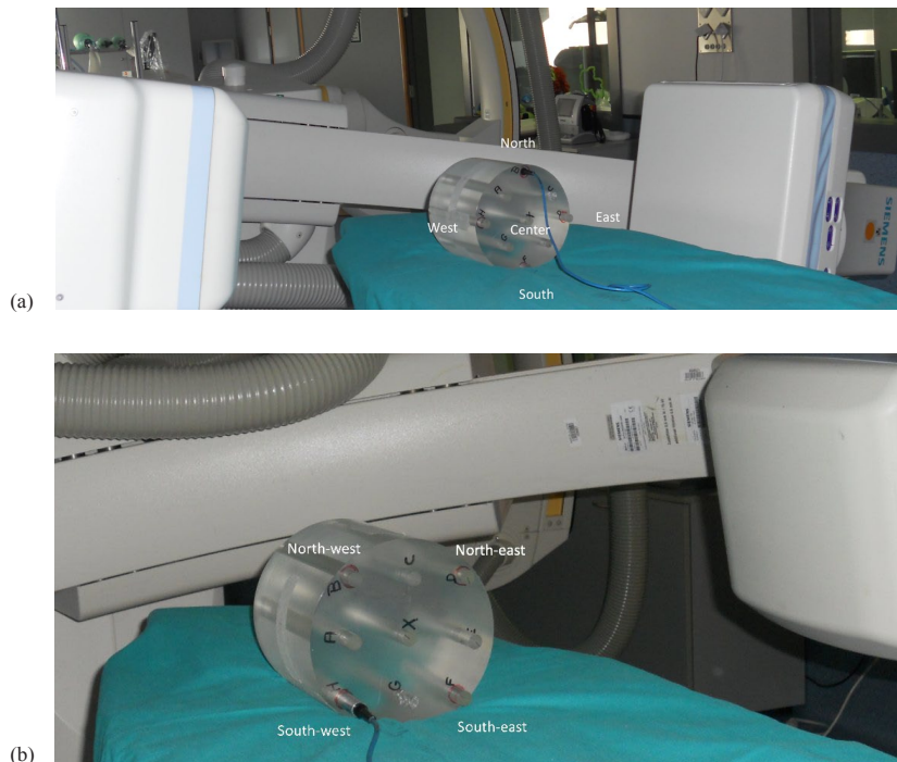
FIG. 3. Perspex CT Radcal model 20CT6 head phantom (a) with a central axial hole to measure the central dose, and four axial holes of the phantom at a depth of 1 cm from the surface to measure the peripheral doses (north, west, south, and east). The phantom was rotated 45° (b) to measure another four peripheral doses (northwest, southwest, southeast, and northeast).
