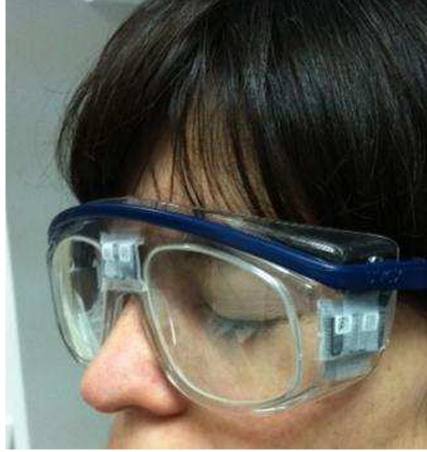
Fig. 3. OSLDs placed on the cardiologist's goggles, two on the external left side and two in the centre.
