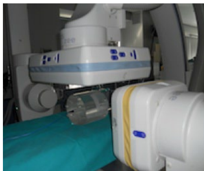
FIG. 4. Biplane acquisition setup using CT head phantom.
