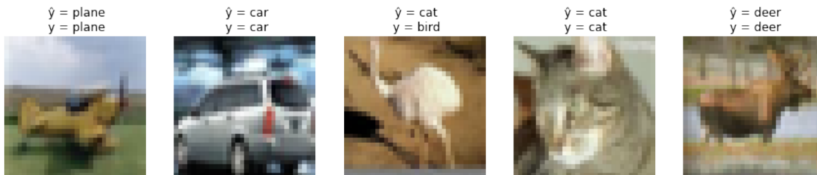
Figure 1.9: Five random samples from the CIFAR-10 dataset and their corresponding predictions and true labels using the VGG architecture. Notice how the convolutional network mistakes an ostrich (bird class) for a cat.
