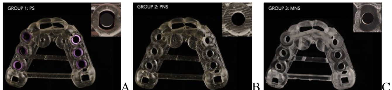
FIGURE 2 | Surgical guides and detail in drill guide tube. (A) PS (additive manufactured—metal sleeve). (B) PNS (additive manufactured—no metal sleeve). (C) MNS (subtractive manufactured—no metal sleeve).
