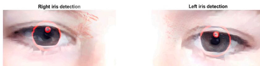
Figure 5. Location of the iris and center of corneal specular reflection.
