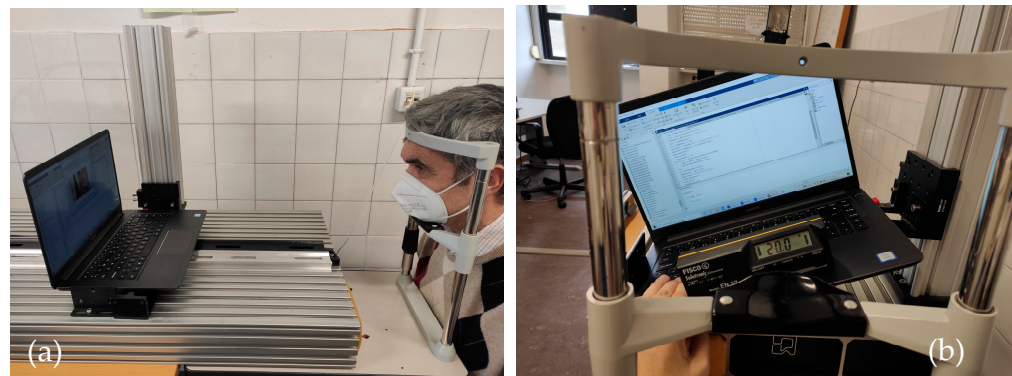
Figure 12. (a). Volunteer with his head resting on a chin rest for the start of the measurement tests. (b) Laptop with inclination controlled by an inclinometer to conduct the tests.
