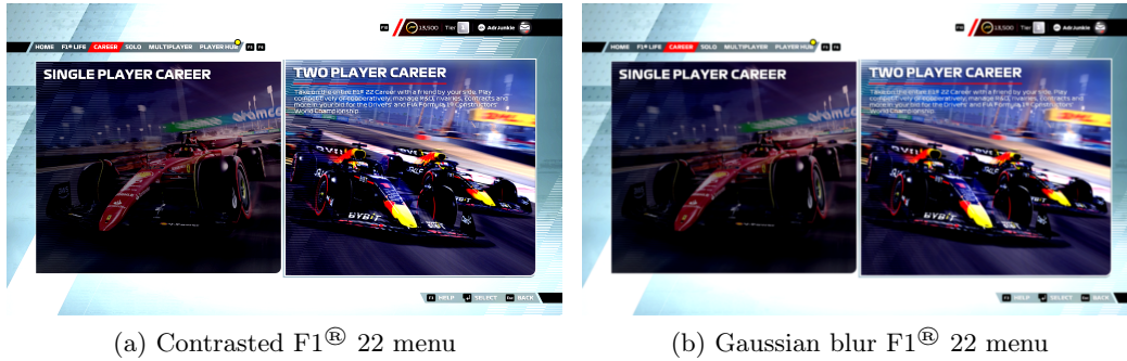
Figure 3.8: Gaussian filter application on contrasted image, the entire image is blurred in order to obtain the most prominent shapes in the image.
