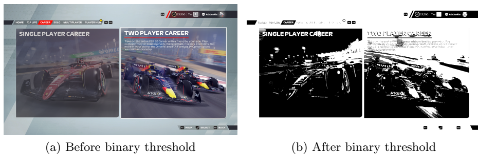
Figure 3.4: F1 ® 22 menu before and after binary threshold
