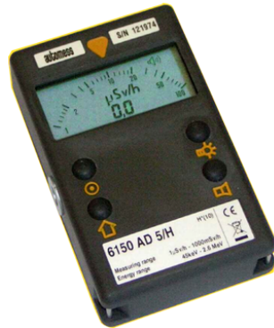
Figure 3.3: Portable dosimeter Automess 6150 AD
