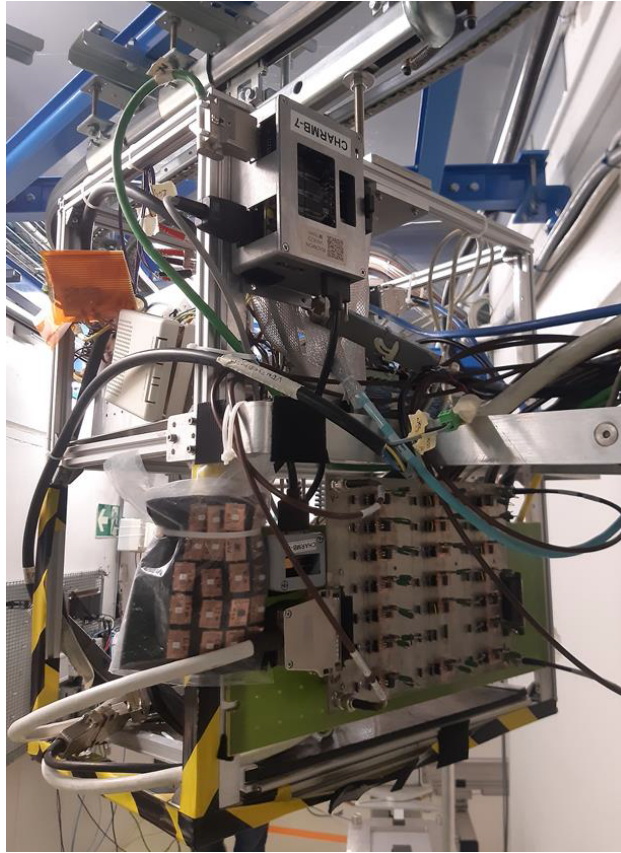
Figure 6.4: Image of the Overhead Conveyor with our setup inside the CHARM facility.
