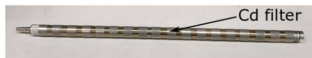
Fig. 7 ^3\text{He} -filled proportional counters are partially covered with 18 cadmium filters (2 cm length and 0.5 mm thickness) in order to physically implement the effect of the composition functions
