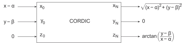
Fig. 6 CORDIC configuration for distance calculation [20].
