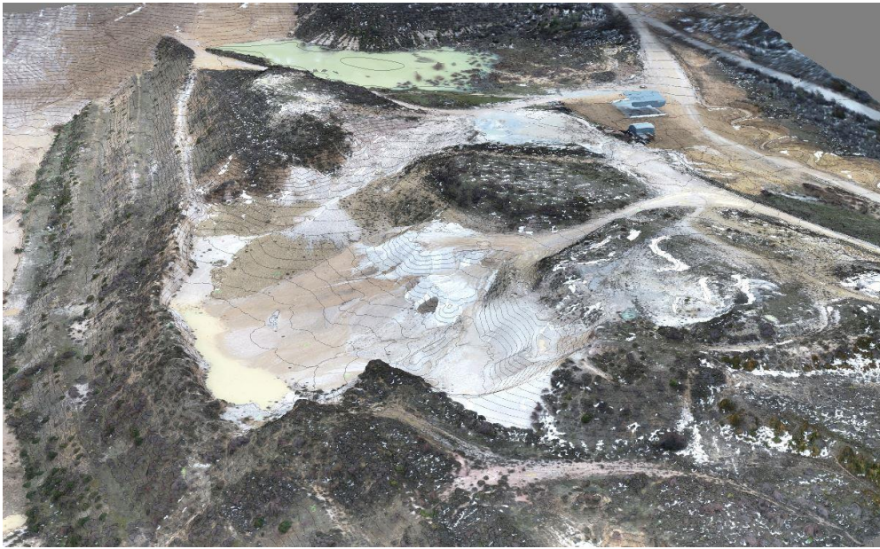
369 Figure 7. Tiled model textured and contour view of the topography surveyed with SfM- 370 UAV on 15.04.2018.
