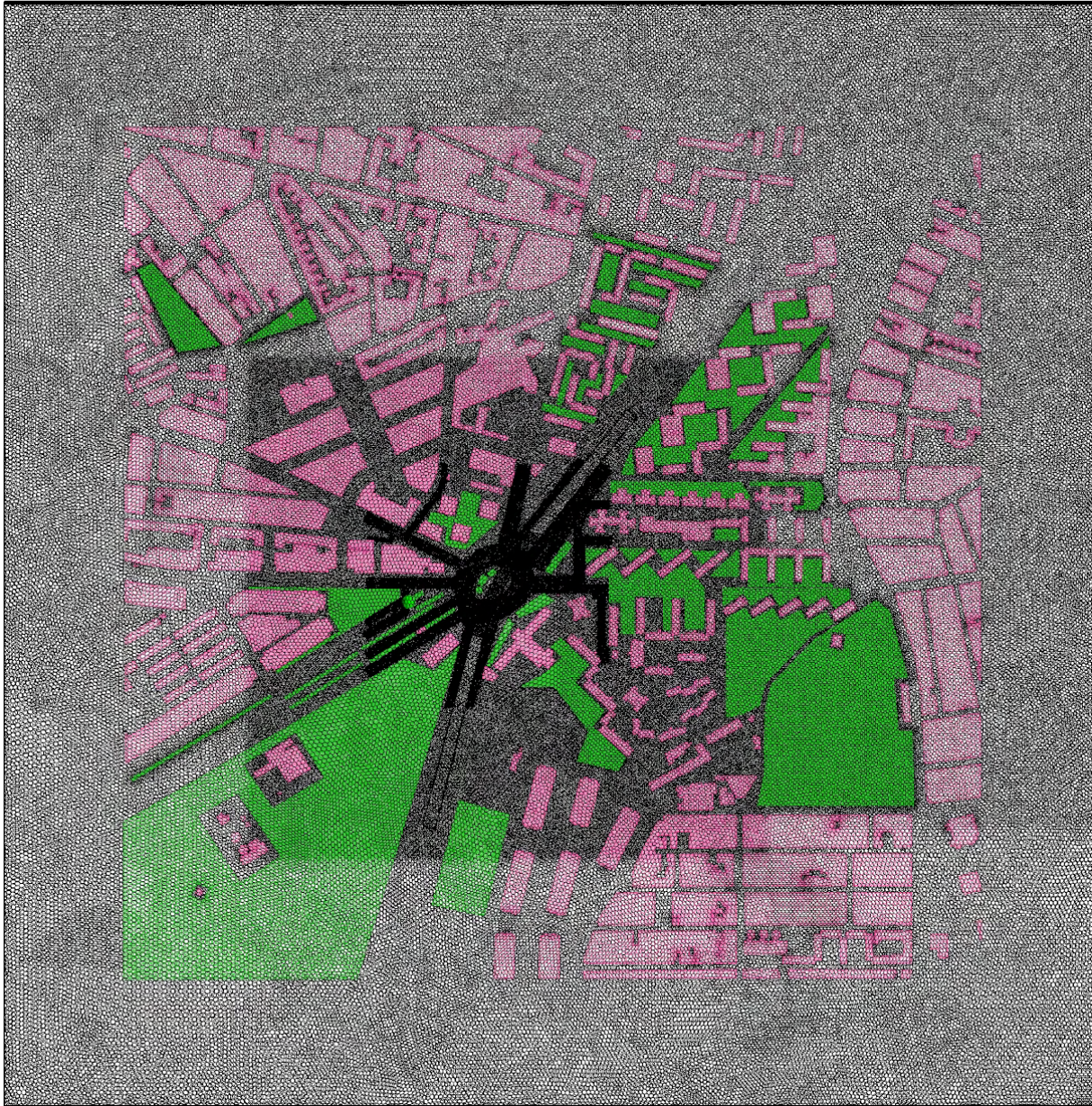
Figure 5.14: Air view of the computational grid. Green cells indicate cells within a vegetation area; pink cells correspond to buildings; and black cells are cells within the air.
