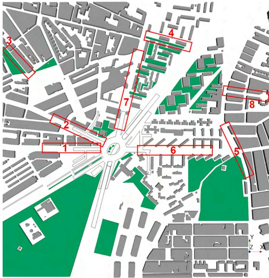
Fig. 5. Domain employed for the CFD model with relevant streets highlighted in red and numbered from 1 to 8. Buildings are coloured in dark grey whereas vegetation is represented with green colour.
