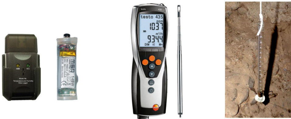
Fig. 6. Measuring instruments: a) Thermo-hygrometer PCE HT-71; b) Thermo-hygrometer MSR 145 W; c) Multifunction meter TESTO 435-2 and hot-wire probe; d) Piche evaporimeter.
