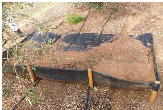
Fig. 2 Design of one of the sediment collection traps implemented in the experimental olive grove in Alentejo (Portugal)
